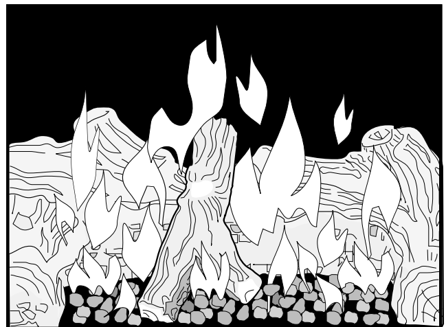
Figure 31. Flame appearance on the "high" setting after approximately 15 to 20 minutes burning.
