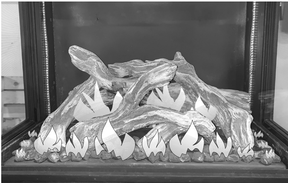
Figure 13.2. Log Set burner flame picture.
