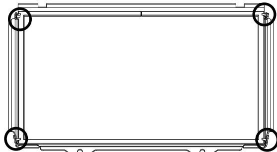
Figure 10.1. Bend the retainer tabs back enough to release the glass panel.
