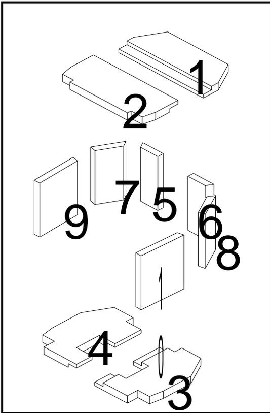
**FIGURE 22. PLACEMENT OF VERMICULITE INSULATION**
