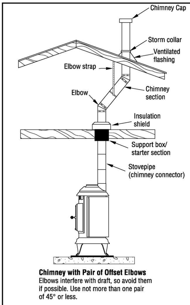
**FIGURE 7. CHIMNEY WITH PAIR OF OFFSET ELBOWS**
