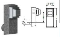
Use for horizontal through-the-wall termination when a vertical rise is desired in the system to meet appliance manufacturer recommended minimum heights. Do not enclose in the wall or install below grade. Provides improved performance in high wind conditions. Features an adjustable air intake and interchangeable shroud (shroud is included and required for all installations). Check with appliance manufacturer for approval and air throttle setting. Patent Pending.
